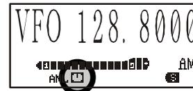
Just press and hold in the **[PWR]** switch for 3 seconds to turn the transceiver back on after an APO shutdown, as usual.
